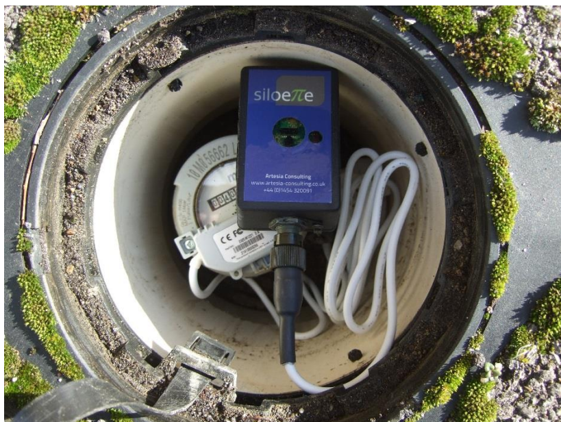
Figure 3 Siloette logger installed in a boundary box
